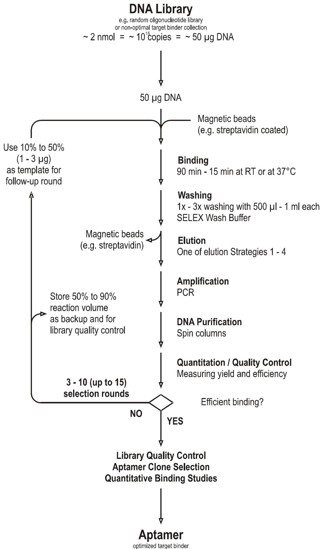
**Figure 4:** From library to aptamer: Schematic overview of the DNA-SELEX work flow. SELEX is a cyclic process. Each completed cyclic sequence of subsequent reaction steps is referred to as “selection round”.
