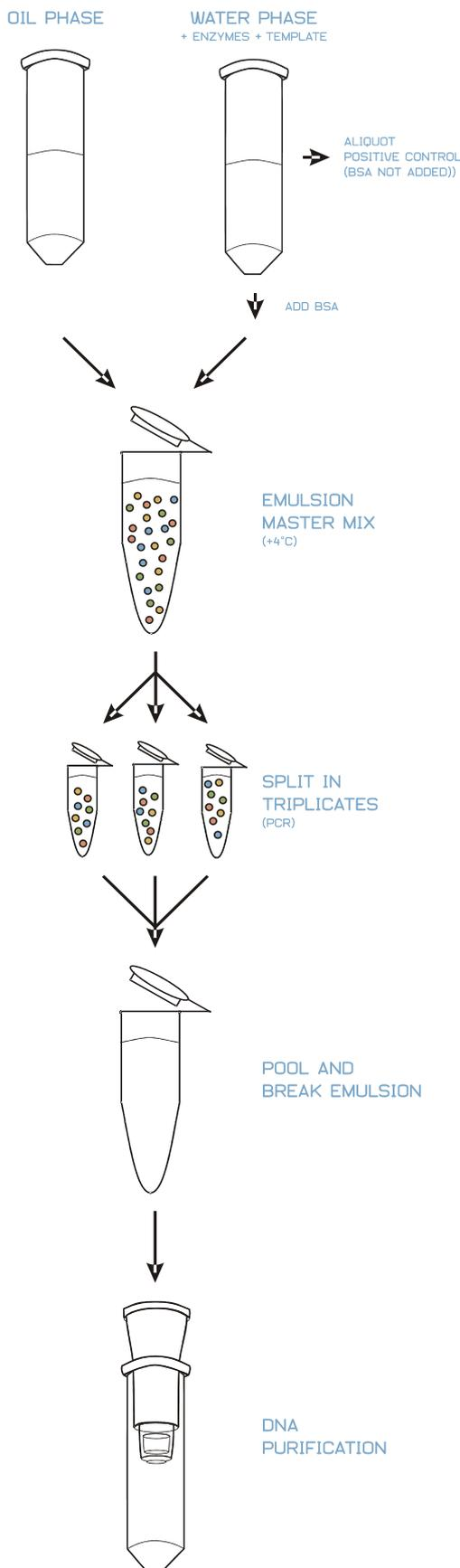
**Figure 6:** General work flow for emulsion PCR (ePCR). Sample volume of the water phase is 50  $\mu$ l. Total reaction volume increases due to addition of the oil phase. Thus, for thermocontrolled reaction conditions (e.g. ePCR), the total reaction volume is split into triplicates.
