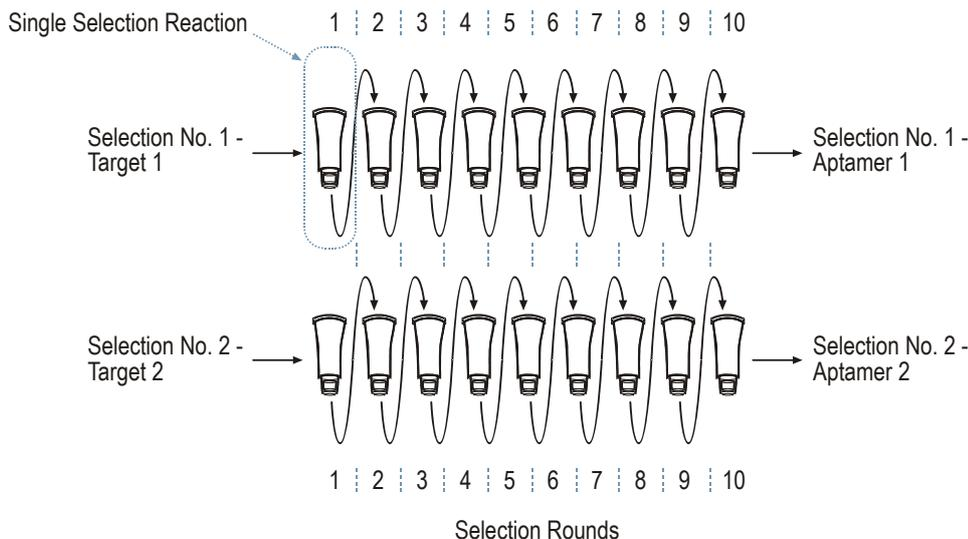
**Figure 2:** Parallel processing of aptamer selection rounds against different targets. The optional use of semi-automated laboratory equipment enables simultaneous high throughput selections against various targets (see Schütze T. *et al.* (2011) PLoS ONE 6 (12) e29604 for further information).
